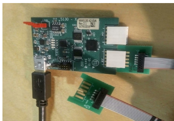
Figure 22 Ribbon Cable Between Driver Board and RF Board
