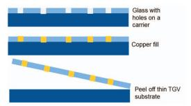
**Figure 10:** Cartoon of leveraging ALoT technology to metallize through vias in 100 um thick glass.
