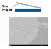
**Figure 13:** SEM image of bottom of metallized via after de-bond (no polishing).
