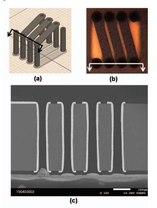
**Figure 4:** 3D TGV inductor formation. (a) 3D rendering, (b) top-down photograph, (c) cross-sectional SEM of TGV with conformal Cu plating on the TGV sidewalls and the top & bottom sides of the glass to form a 3D TGV inductor
