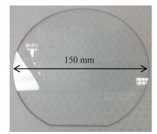
**Figure 11:** Image 100 um thick glass with 30 um diameter vias temporarily bonded onto a glass carrier using ALoT technology.
