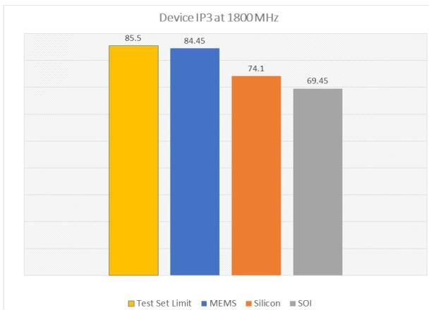
Fig. 8. IP3 for MEMS and other technologies
