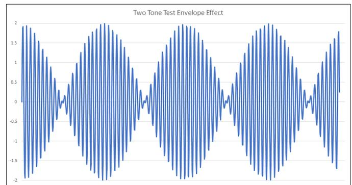
Fig. 3. The envelope effect shown by adding two high-frequency signals creating a low-frequency component or beat frequency
