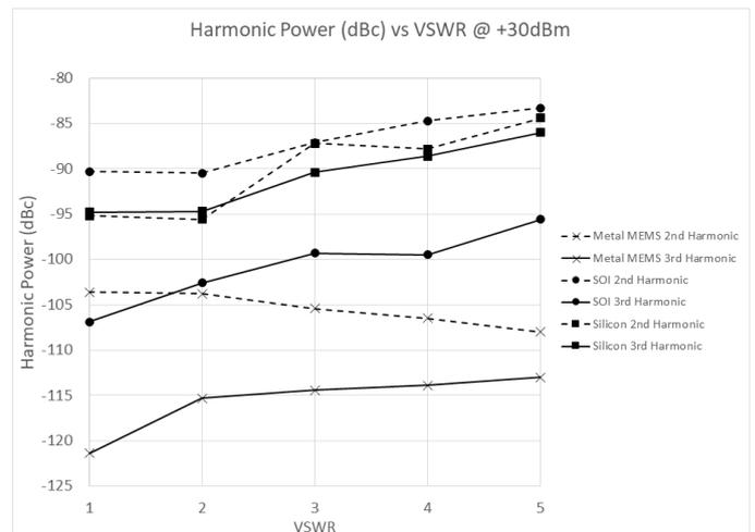
Fig. 6 Harmonic response power relative to carrier against VSWR
