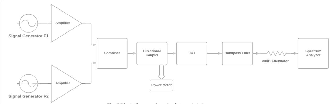
Fig. 7 Block diagram of passive intermodulation test setup
