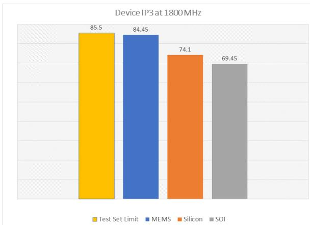
Fig. 8. IP3 for MEMS and other technologies
