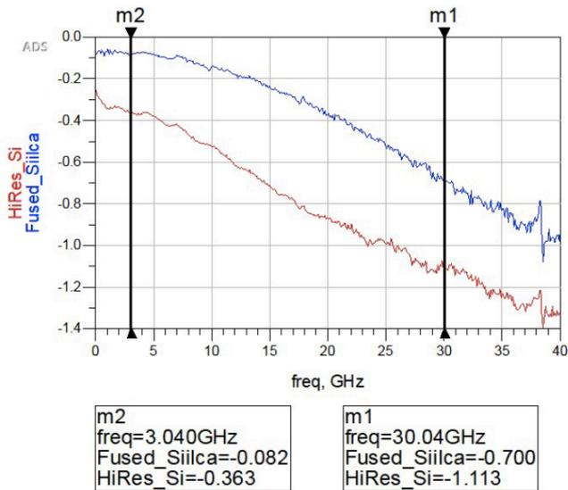
Fig. 2. Measurement results of the same layout built on fused silica (Red Line) and 3000  $\Omega$ -cm Si (Blue Line) substrate.
