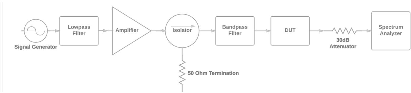
Fig. 4 Block diagram of benchtop harmonic response test set up
