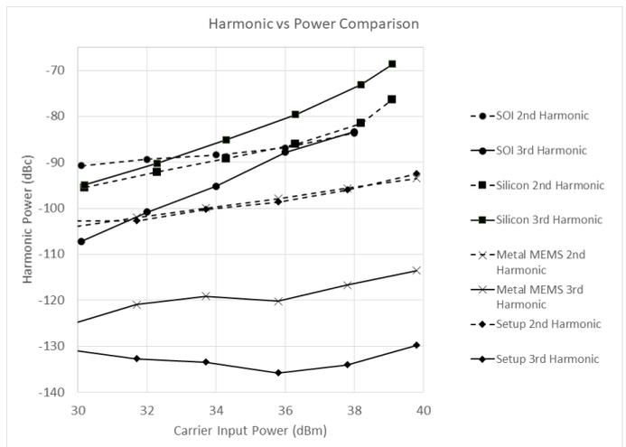
Fig. 5 Harmonic response power relative to carrier against input power level
