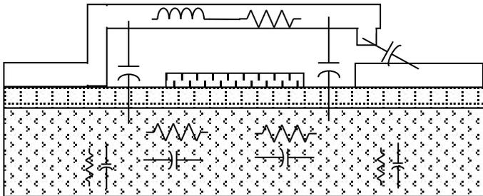
Fig. 1. The parasitic elements around MEMS substrate and in the substrate.
