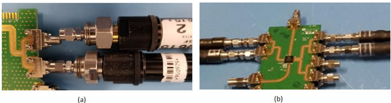
Figure 20. (a) Cable cannot be plugged (b) Cable can be plugged directly
