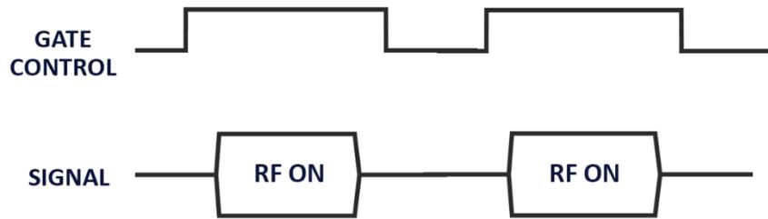
If the MM3100 is used in hot switching applications, the number cycling operations of the device will be degraded. See section [Switch Reliability Test Results](#) and [Figure 13](#) for more information.
