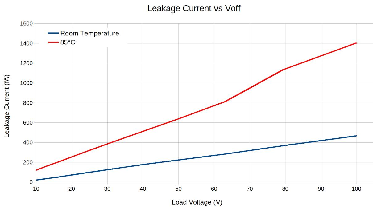
**Figure 9. Off-State Input-Output Leakage Current vs  $V_{OFF}$**
