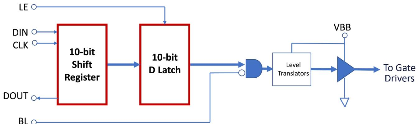
**Figure 14. High-Voltage Gate Driver Block Diagram**
