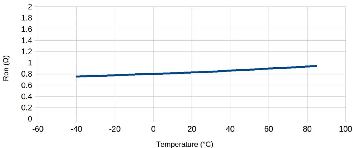
**Figure 8. On-State Resistance over Temperature**
