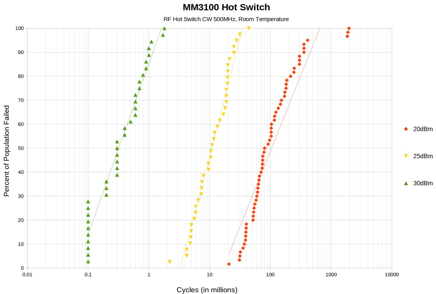
**Figure 13. Hot Switch Endurance Test Results**
