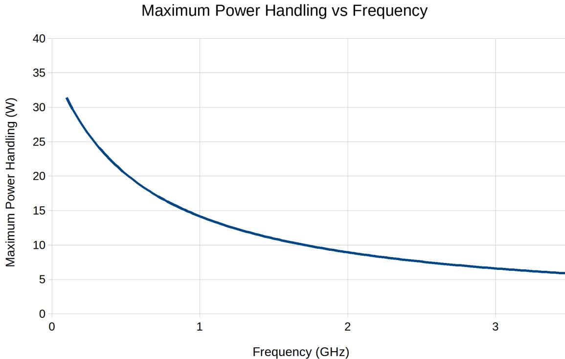
**Figure 4. Maximum Power Handling versus Frequency at Ambient 45°C**
