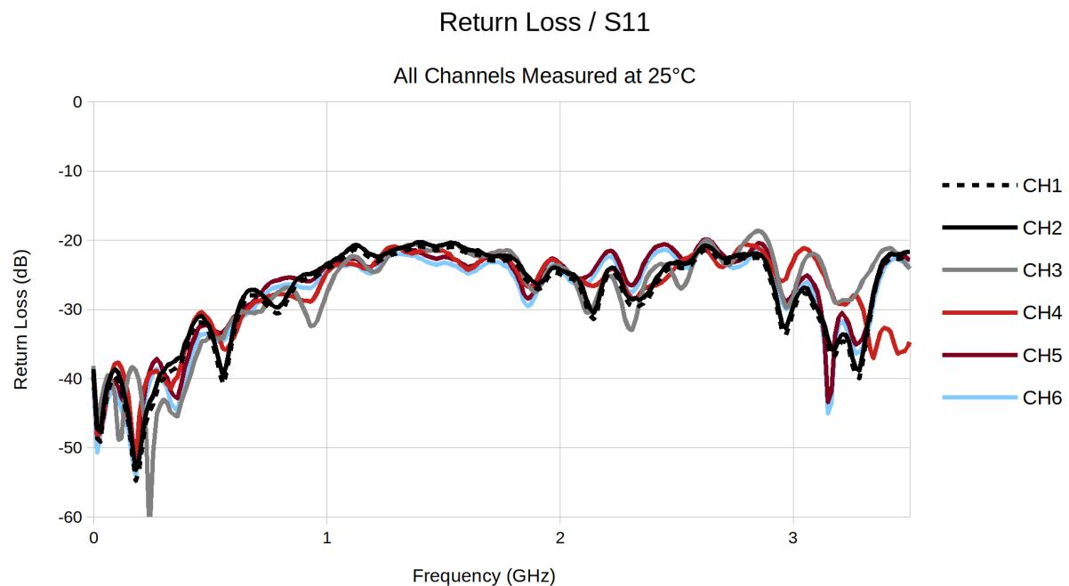
**Figure 11. Typical Return Loss vs Frequency (S<sub>11</sub>)**
