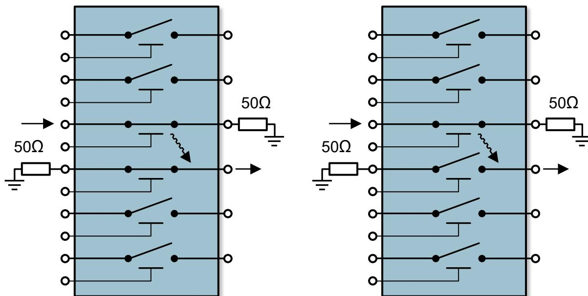
**Figure 7. Adjacent Channel Isolation Measurement**
