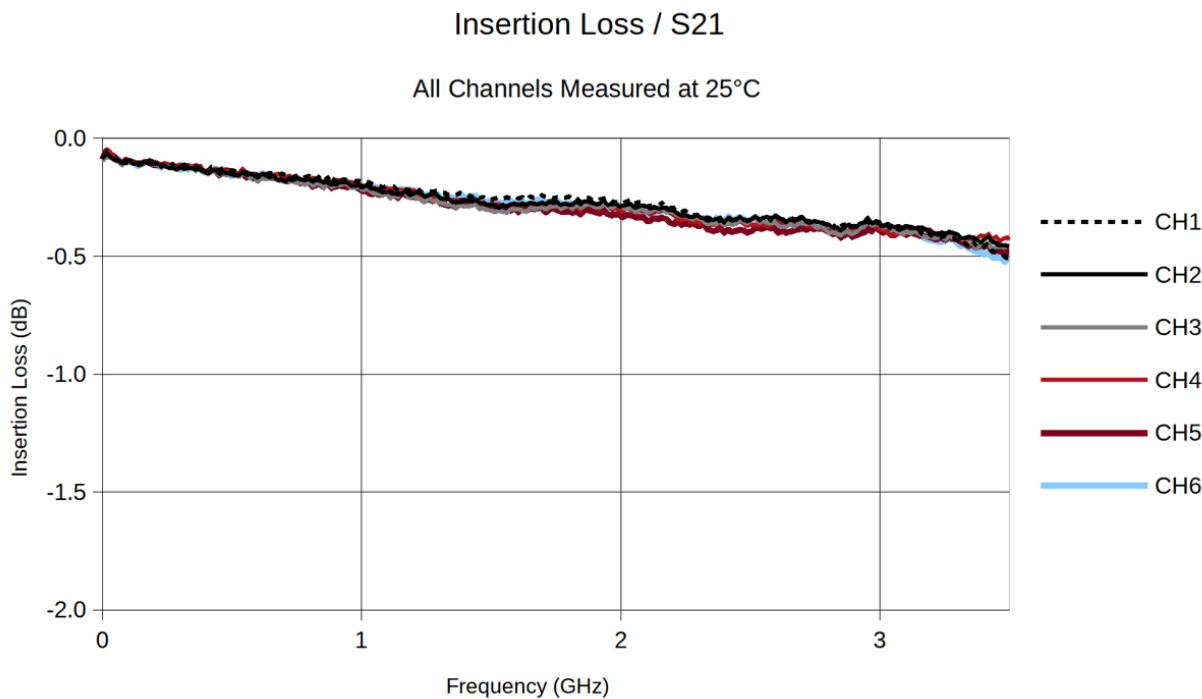
**Figure 10. Typical Channel Insertion Loss vs Frequency (S<sub>21</sub>)**
