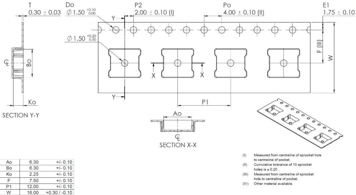
**Figure 19. Tape and Reel Drawing**
