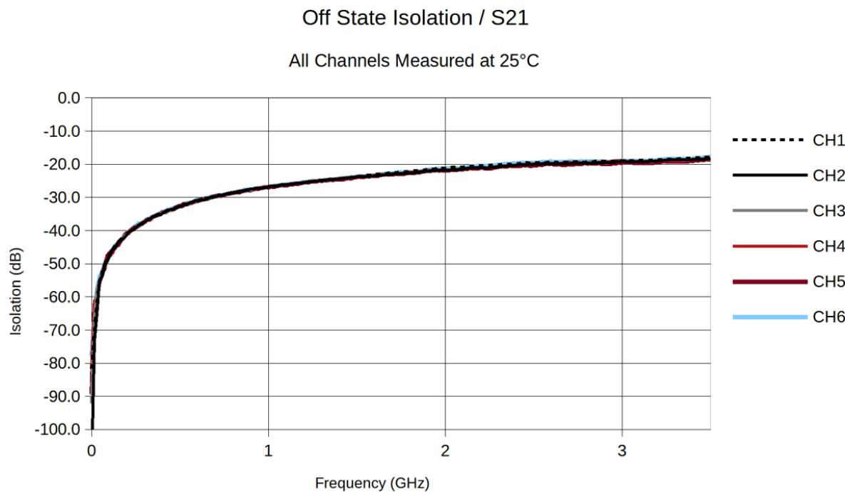
**Figure 12. Typical Input to Output Isolation vs Frequency (S<sub>21</sub> with channel off / open)**
