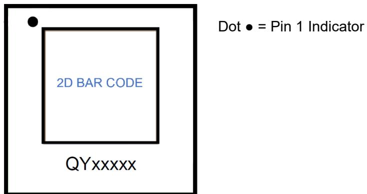
**Figure 18. Package Marking Drawing**
