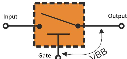
**Figure 3. Open Switch Gate ( $V_{BB}$ ) to Output Voltage Considerations**
