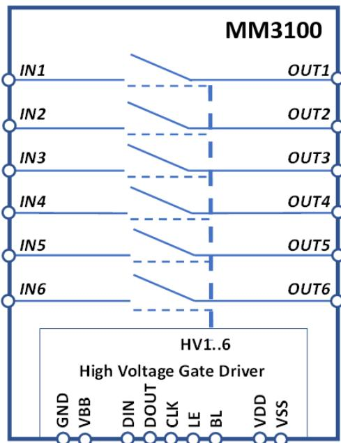
**Figure 5. Functional Block Diagram**
