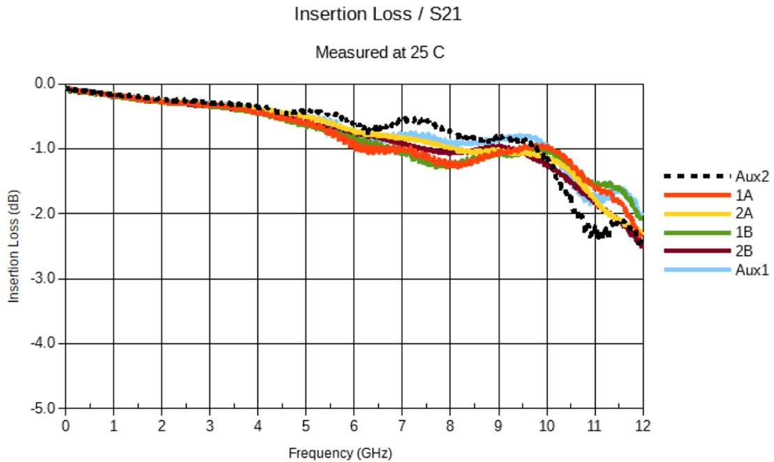
**Figure 5. Single-ended Insertion Loss / S21**
