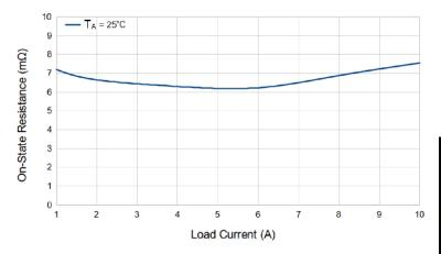
1P1S Configuration at 10 Amps with 7.6 m $\Omega$
