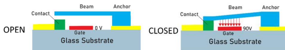
Figure 1: Cross-Section Diagram of MEMS Switch with gate line; 0V = OFF and 90V = ON
