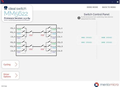
6. To connect the HS1\_A/HS1\_B port to the HS2\_A/HS2\_B port, click on the "HVA" and "HVB" switches.
