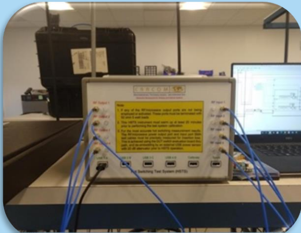
Menlo Micro's custom-designed RF hot-switch tester (4 ch, 33dBm, 6GHz)
